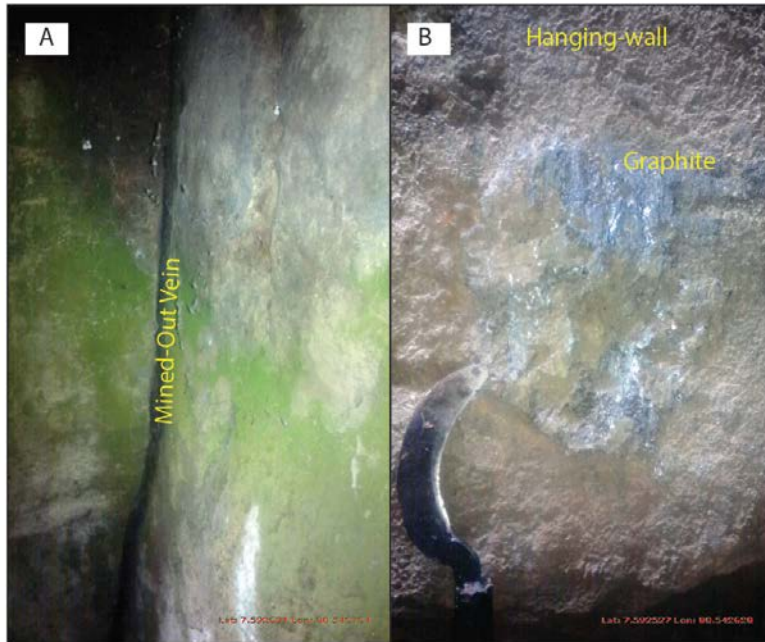
Figure 2-2: Occurrence of graphite veins in historical workings. Vein 1 (A); and, Vein 2 (B).
