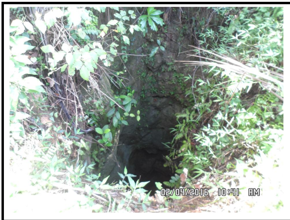
Plate – I: A partly filled shaft structure in an abandoned graphite mine within the selected grid unit
