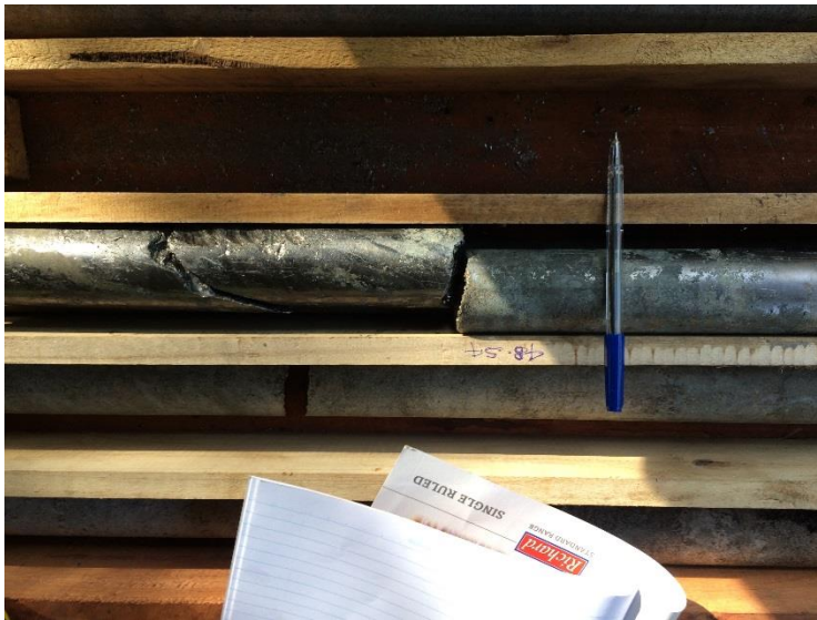
Fig5.2 The graphite vein (30cm) was identified from bore hole number DH001
