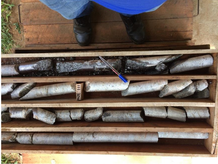
Fig 5.1 The graphite vein (60cm) was identified from bore hole number DH003
